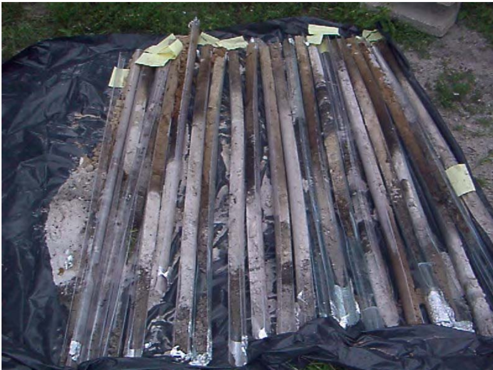
Photo 2: Core borings from monitoring wells show natural soil variations and variations due to fill.
