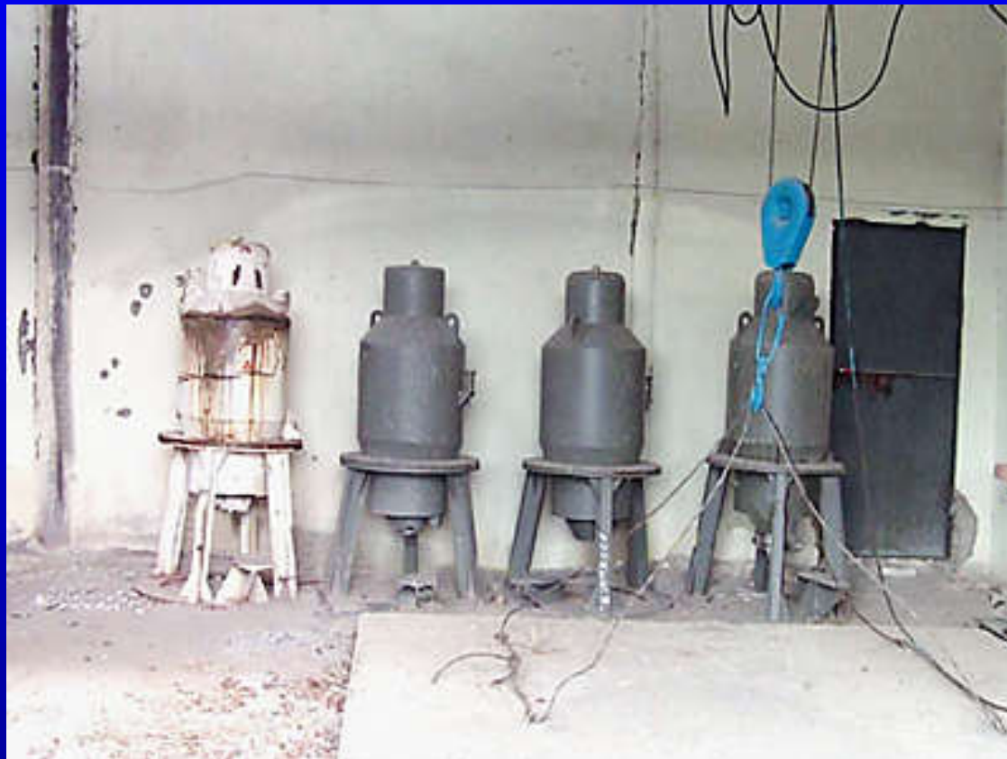
Sources used in mobile cesium irradiators in the former Soviet Union
