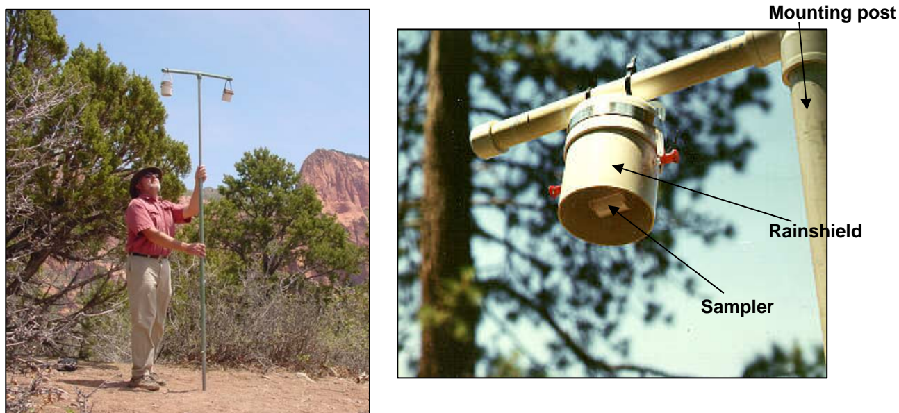
Figure 4-1. Typical Integrated Passive Ozone Monitoring Station and Close-up of Sampler and Rainshield.
