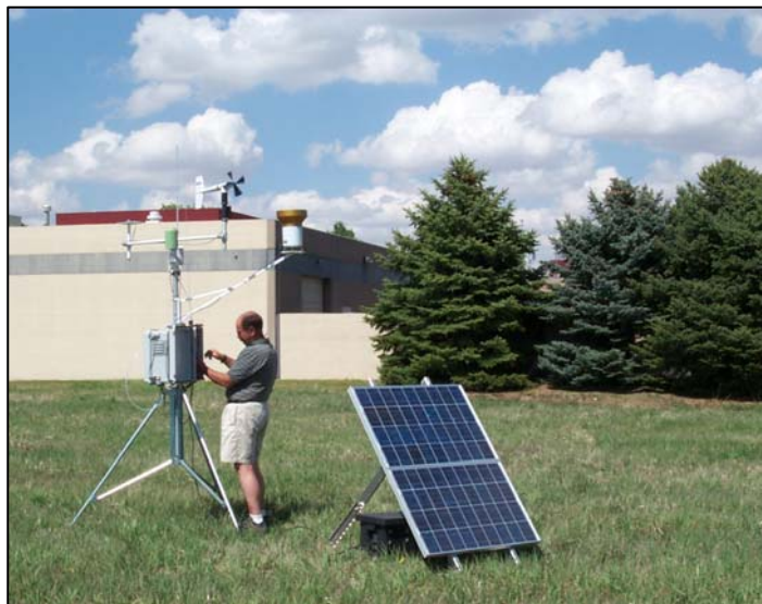
Figure 3-1. Typical Portable Continuous Ozone Monitoring Station.
