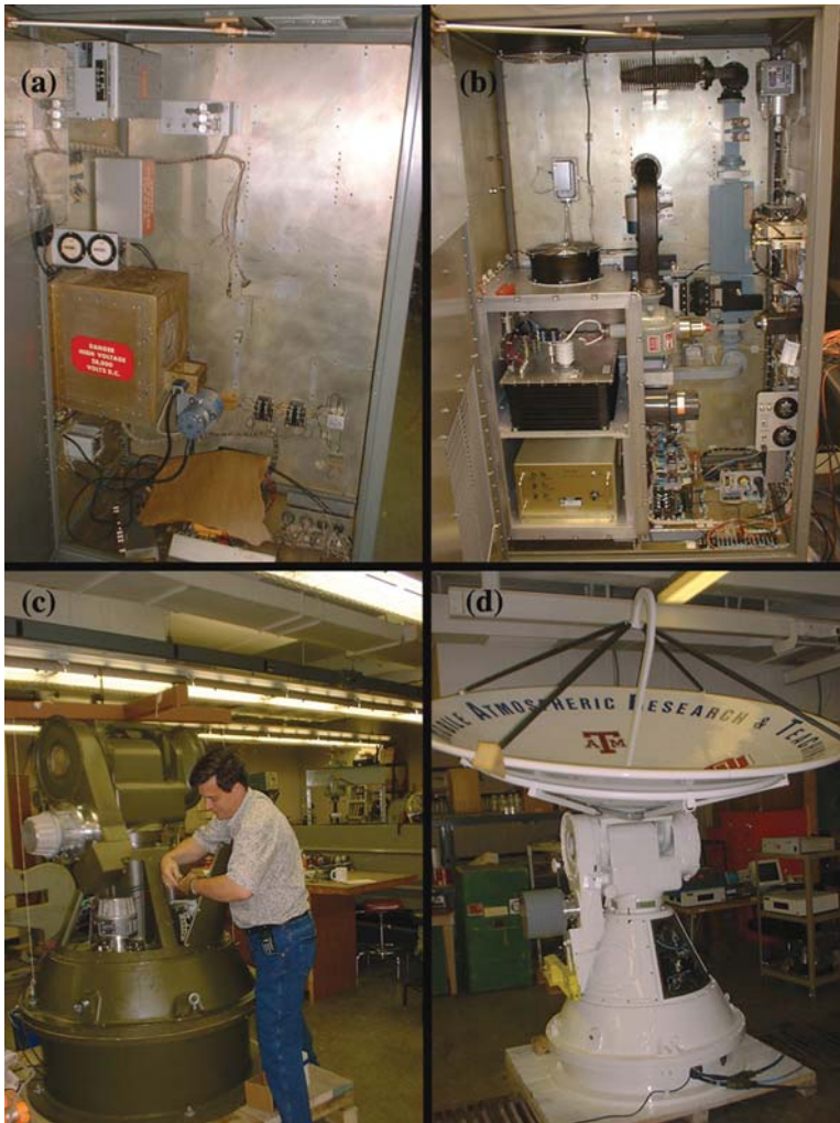
FIG. 2. Inside view of the SMART radar transmitter a) before and b) after modification. Note the a) original size of the high-voltage cage, identified by the red label, compared to b) the custom-fabricated unit in the lower-left portion of the transmitter cabinet. The high-voltage cage was increased in size by a factor of 2 to accommodate the new solid-state modulator and high-voltage power supply. c) The World War II era cast-iron pedestal was refurbished both mechanically and electrically at TAMU by J. Guynes (shown). d) The final product was repainted and integrated with the NWS WSR-74C antenna.
