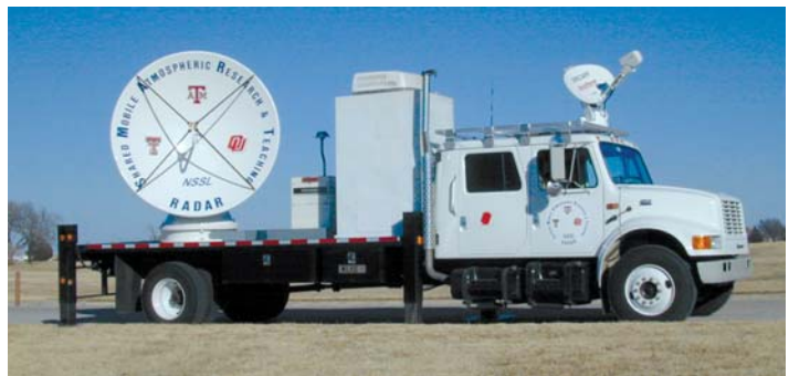
FIG. 1. Side view of SR-1, the first mobile C-band Doppler weather radar in the United States. The smaller dish on top the cab is a self-pointing satellite-based Internet communication system that will allow for the real-time transmission of the data back to a remote server. Photo taken at NSSL where the SMART radars are housed. View is to the east-northeast.
