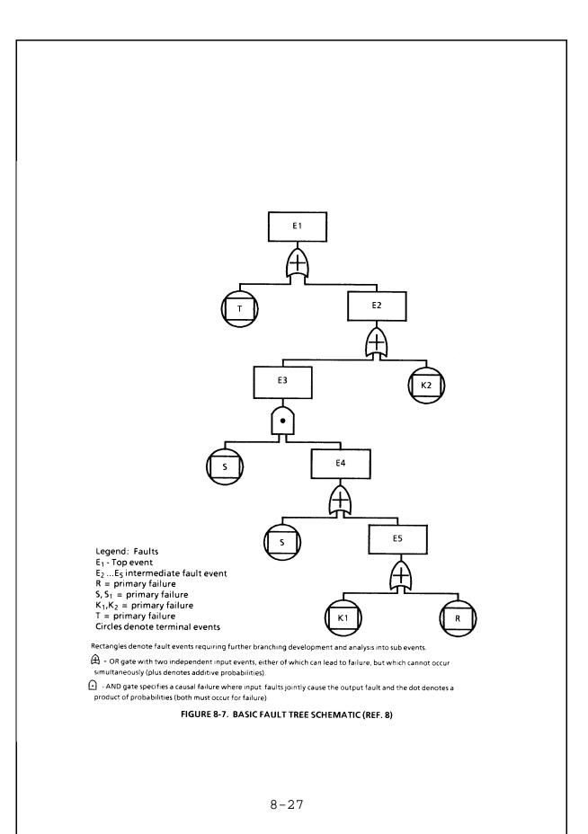
The AND gate represents the simultaneous occurrence of conditions or events necessary to result in failure propagation up the tree. An OR gate indicates that each individual failure event entering is capable of leading to higher level failures. Careful consideration must be given to the independence or mutual interdependence of events entering a particular logic gate to insure the correct use of joint and conditional probability concepts.
