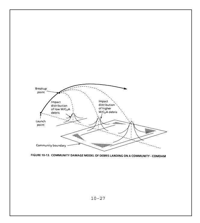
The model is deterministic, not probabilistic (see Ch. 8), i.e., given a catastrophic ELV failure and the absence of a destruct system, it examines the nature and severity of possible consequences of interest, namely a conditional casualty expectation. In reality, implementation of Range Safety restricts launch azimuths as well as decreasing the likelihood of any accident that could have public impacts (see Ch.9).
