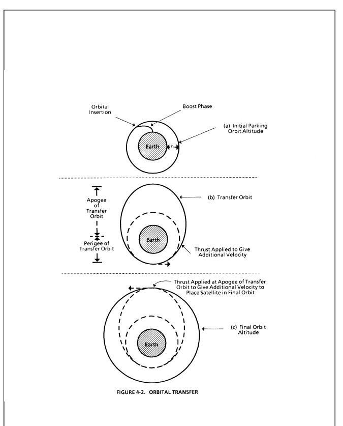
elliptical orbit indefinitely, passing (ideally) through its initial perigee point once very revolution. If the objective is to reach a higher circular orbit, the built-in rockets (apogee kick motors, AKM) can be fired again (for a specified period of time) when the satellite reaches the apogee of the elliptical orbit, and the new orbit will be as shown in Figure 4-2(c).
