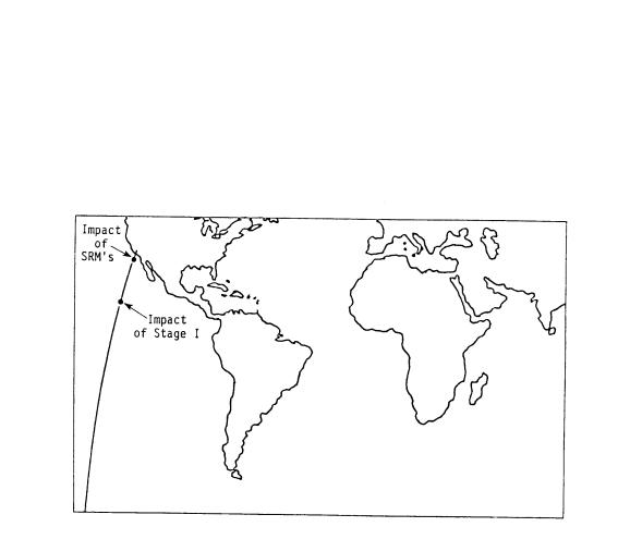
FIGURE 10-7. LOCUS OF IIP FOR A TYPICAL TITAN III LAUNCH FROM VANDENBERG AIR FORCE BASE (WTR)
