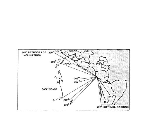
FIGURE 10-8. WTR GEOGRAPHIC LAUNCH AZIMUTH CONSTRAINTS (REF. 7)
