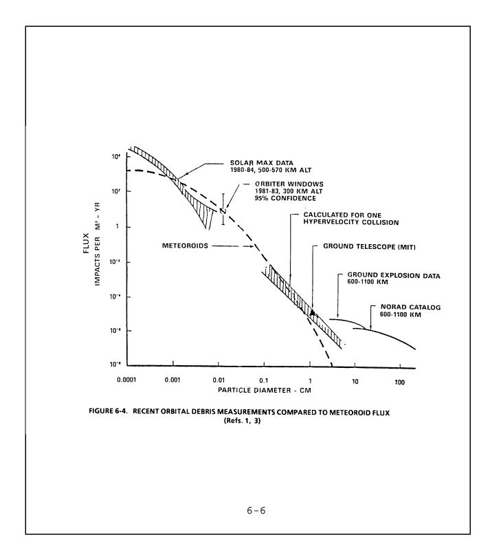
Untracked smaller debris appear to dominate collision encounters. Little data on the man-made debris flux are available on debris less than 4 centimeters in size (Fig.6-1). Objects below this size cannot be detected by Space Command's deep space tracking detection systems. GEODDS (The Ground-Based Electro-Optical Deep Space Surveillance System) however, is an expanding global network of tracking sensors which is continually being upgraded to aid in monitoring space assets.<sup>(13)</sup>
