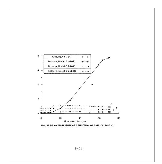
In Fig. 5-6, the hazard distances first increase with time, and then decrease -- following the behavior of the potential explosive energy profile which is shown in Fig. 5-5. Furthermore, Fig. 5-6 can be interpreted as follows:
