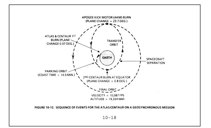
However, even if the mission fails to insert the payload into the correct final orbit, public hazards may not increase unless a highly elliptical transfer orbit leads to early uncontrolled reentry of upper stages and payload or an on-orbit explosion creates collision hazards for GEO and LEO operational satellites.
