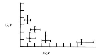
(a) Plotting of points corresponding to individual failure events. Logarithmic scales usually used because of wide range in values. The error brackets denote uncertainties in probability estimates (vertical) and in anticipated consequences (horizontal) for each failure mode/event.
