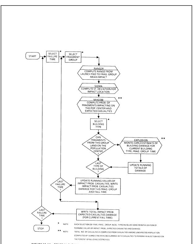
FIGURE 10-14. GENERAL FLOW DIAGRAM OF COMMUNITY DAMAGE MODEL, COMDAM
