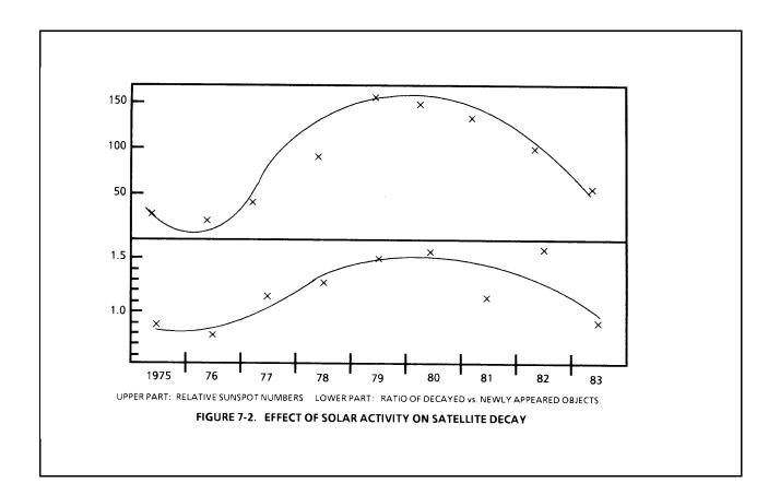
During the past 5 years there have been an annual average of 548 decays from lower altitude orbits (i.e., about three satellites re-entering every 2 days). Almost 83 percent of Earth satellites reside in LEO orbits (see Chapter 6) with periods of less than 225 min (about 4 hrs) and are near term re-entry candidates (see Figs.4-3 and 7-1). The total number of satellite decays per year is shown in Figure 7-3.  $^{(11)}$
