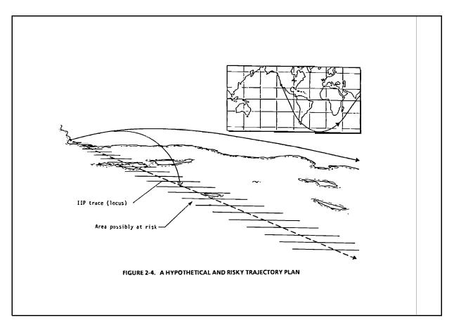
risk analyses are performed using models that consider the probability of the vehicle failing in a variety of modes and simulate the behavior of the missile during and after malfunction, including the effect of activating the flight termination system.
