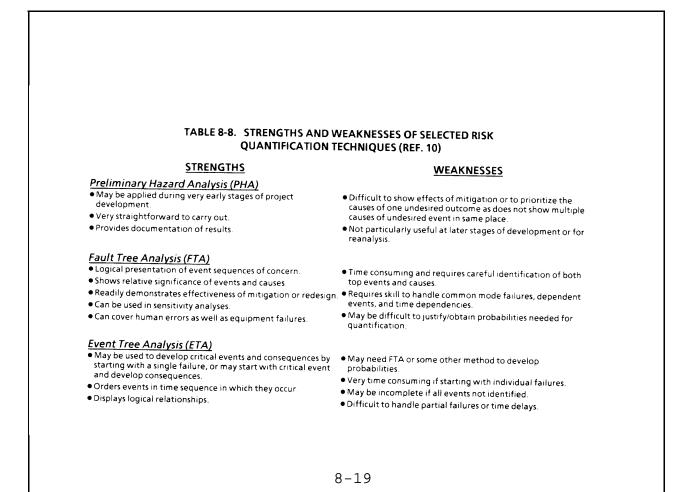
There are several inductive methods of risk analysis which assume a particular failure mode or failure initiating event. The effects on the system performance are then analyzed in order to infer the propagation of failures (failure chains) and to assess the sensitivity of the system operation to the postulated initial failures (bottom to top). The methods listed below focus primarily on hazard identification and on the probabilities of occurrence of hazardous events:
