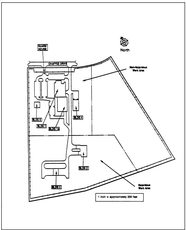
Building 1A, the later addition, contains one clean room high bay with its own clean room airlock. The overall building dimensions are 95 feet x 170 feet x 60 feet. Both buildings are constructed of steel columns and beams with metal stud framing, except for the office and support sections of Building 1, which are of concrete masonry block.
