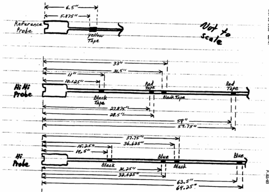
Figure 5.3 - Tape reference points on leads to the HIGH and HIGH-HIGH Warrick Conductivity Sensors (as Provided by AmerenUE)
