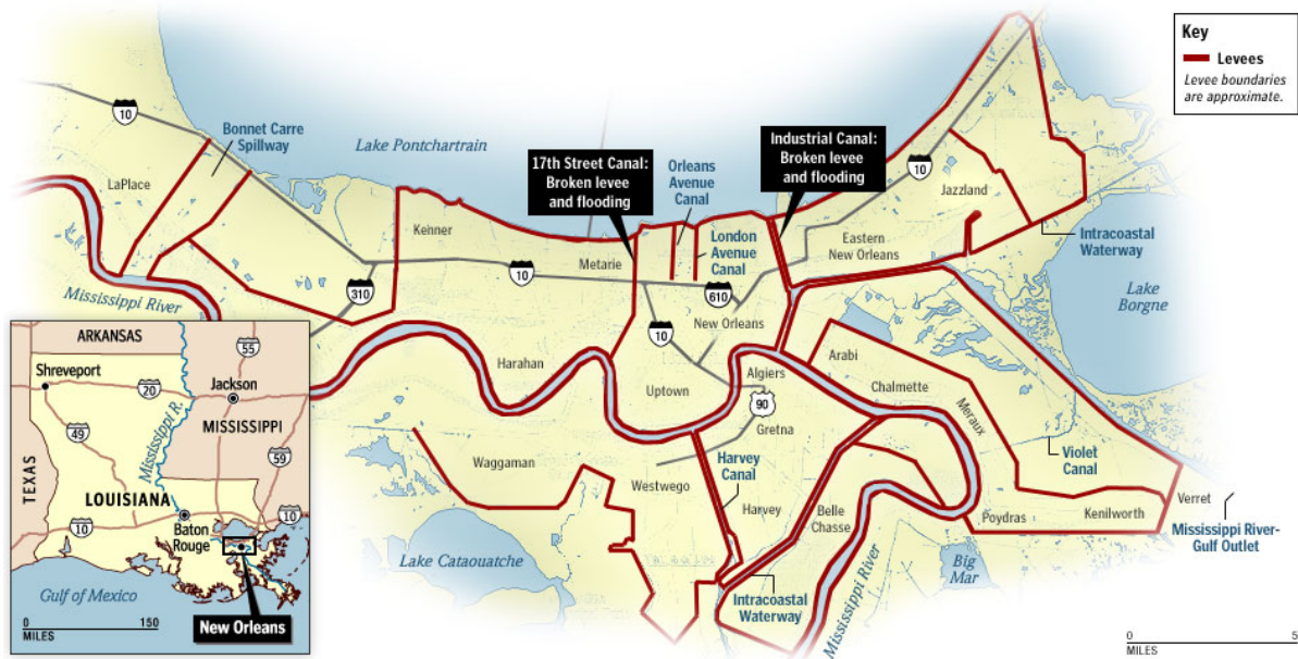
Figure 5. Map of New Orleans Levees and Locations of Major Levee Breaches After Hurricane Katrina
