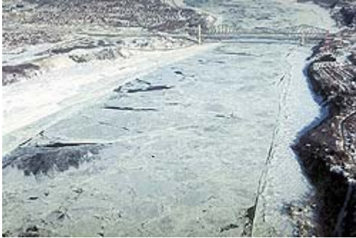
Photo 1.7: View of Quebec City bridges with nilas and grey ice mixed with thin brash moving down under the bridge. Extensive fast ice (battures) has formed on both sides of the river.
