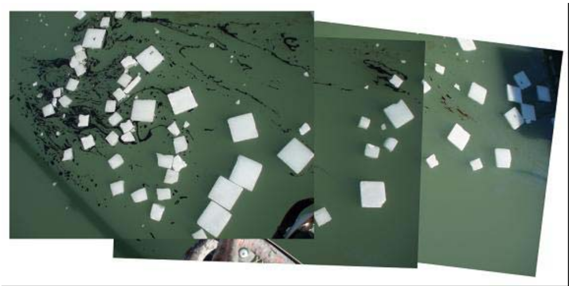
Figure 25: Overhead picture of Test 2 at end – note small slicklets.
