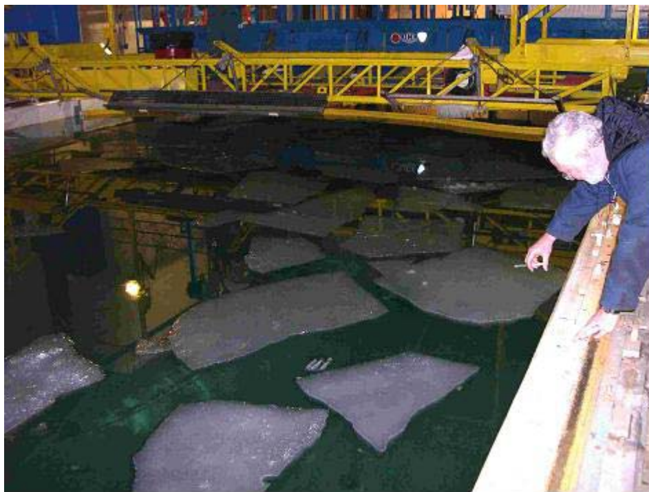
Figure 10: Applying herder around periphery of slick.
