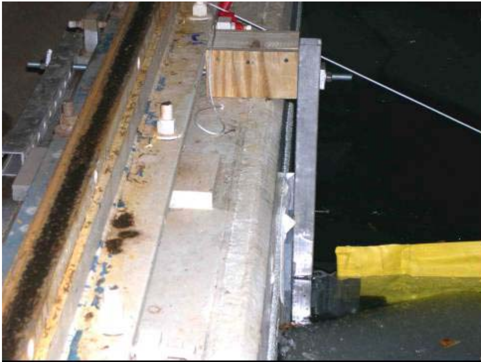
Figure 3: Custom designed boom clamp to seal boom against basin wall.
