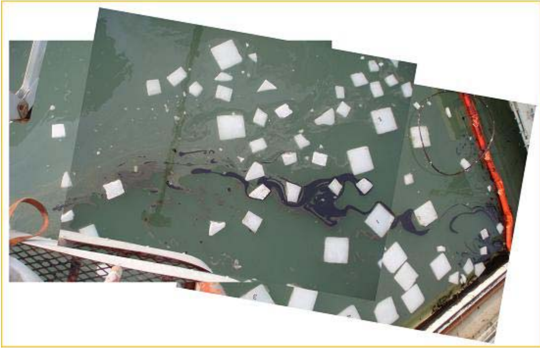
Figure 31: Test 5, six minutes after herder applied.
