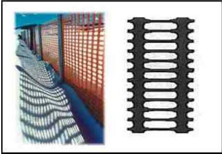
Figure 36: Plastic snow fence material used to construct windbreak around test pool.
