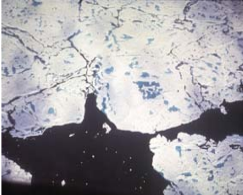
Photo 1.4: Large pans of old ice showing secondary drainage pattern and puddling
