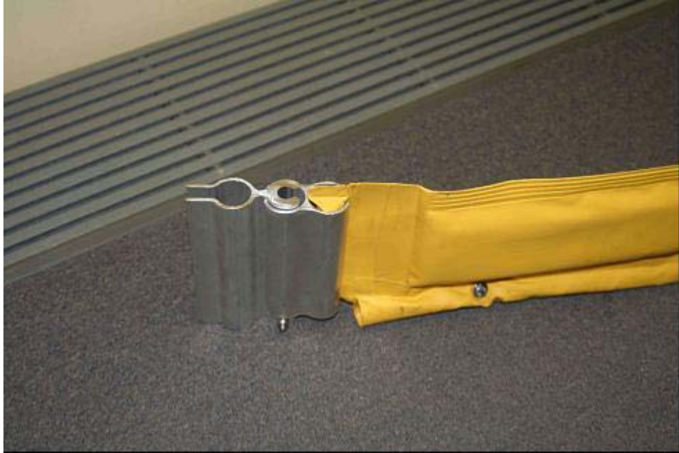
Figure 2: Specially built small oil boom and slide connector to divide basin into test areas.
