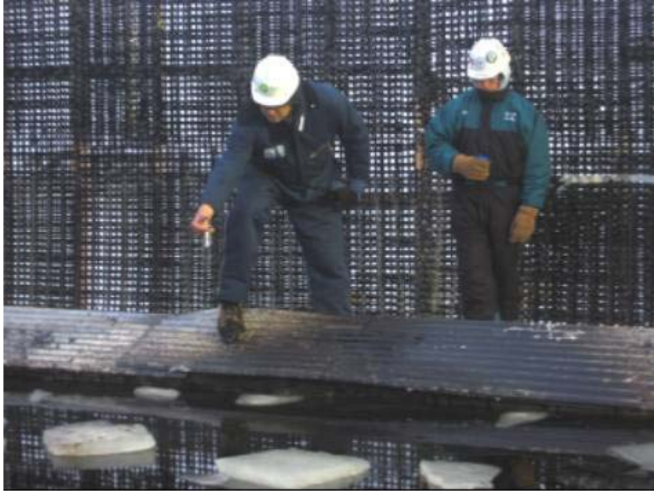
Figure 42: Adding herder dropwise from syringe around periphery of test pool.
