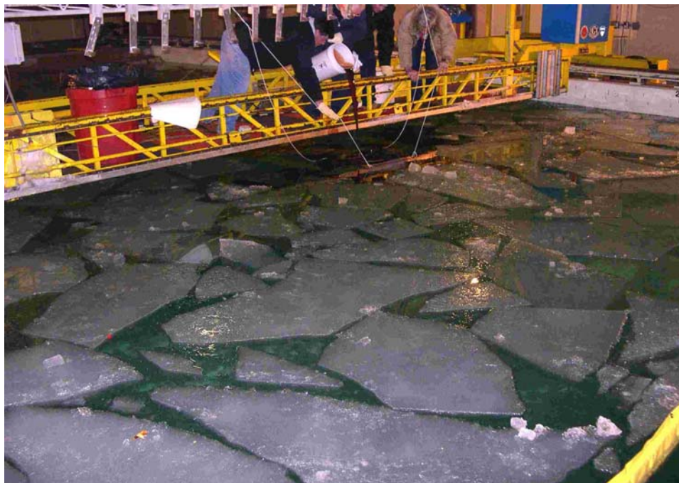
Figure 5: Oil being poured onto spill plate in test area.
