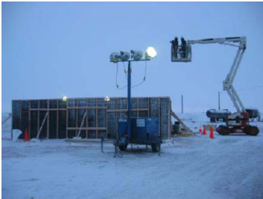
Figure 41: Position of lift basket for digital photos (and video) of oil on test pool.
