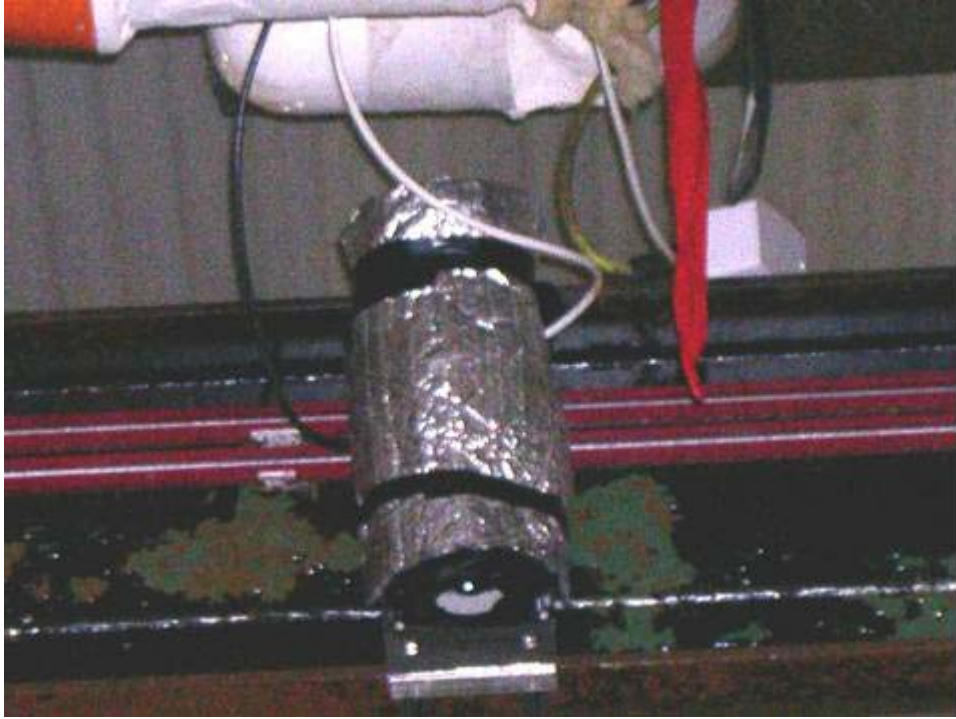
Figure 6: Insulated video camera mounted vertically on beam high above center of test area.
