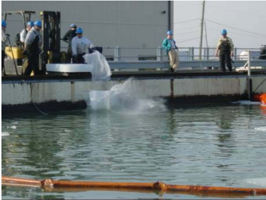
Figure 18: Adding ice slabs to test area.
