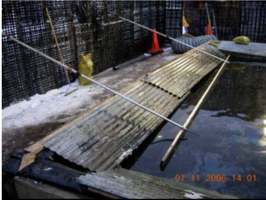
Figure 48: Board and pole arrangement used to generate small waves in test 16 and 17.
