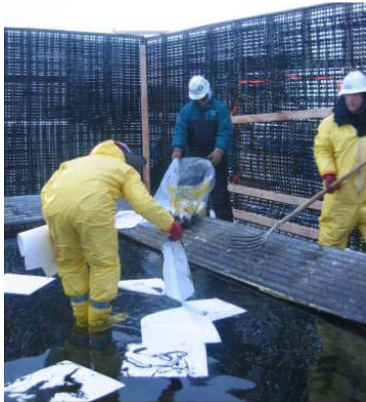
Figure 45: Recovering residue after burn to determine removal efficiency and rate.
