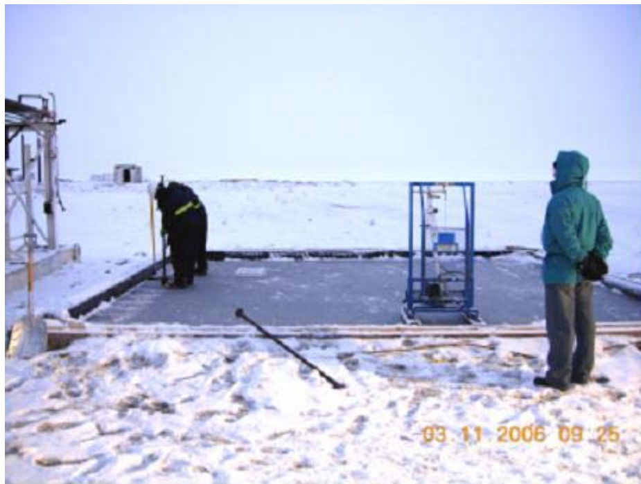
Figure 37: Shallow pit used to grow saline ice used to simulate brash ice in test pool.
