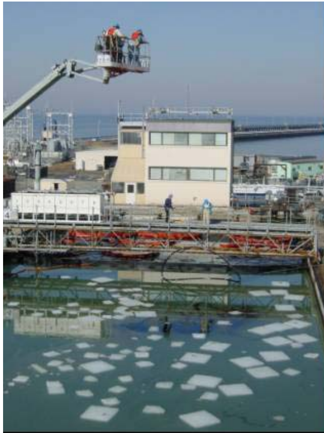
Figure 20: Containment ring lifted to release oil to drift into ice.
