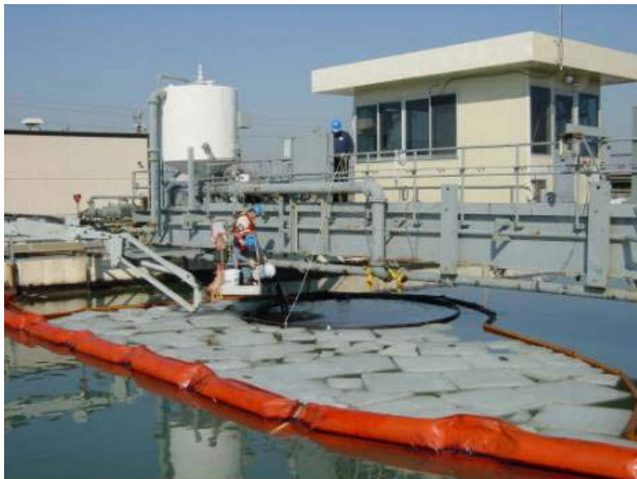
Figure 19: Adding crude oil to containment ring.
