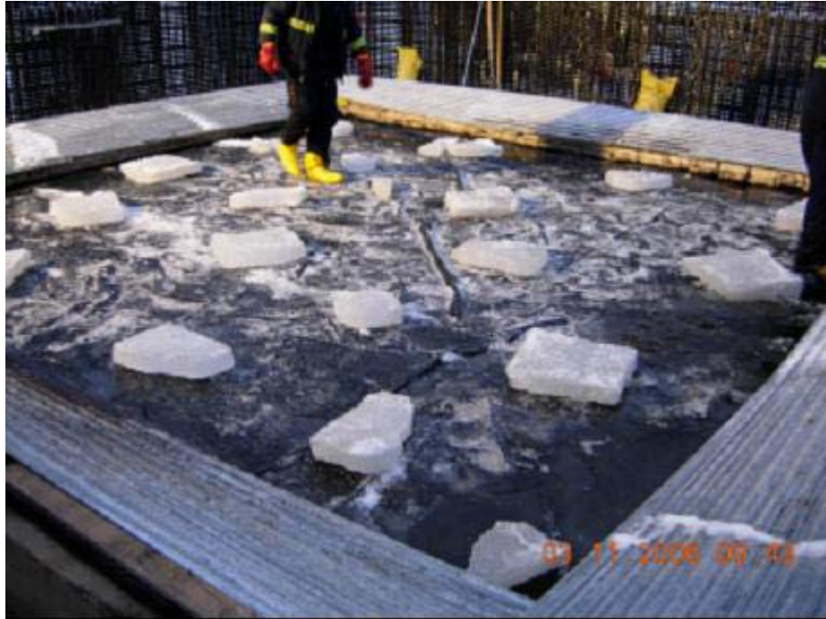
Figure 38: Ice slabs being placed in test pool to simulate 10% brash ice cover.
