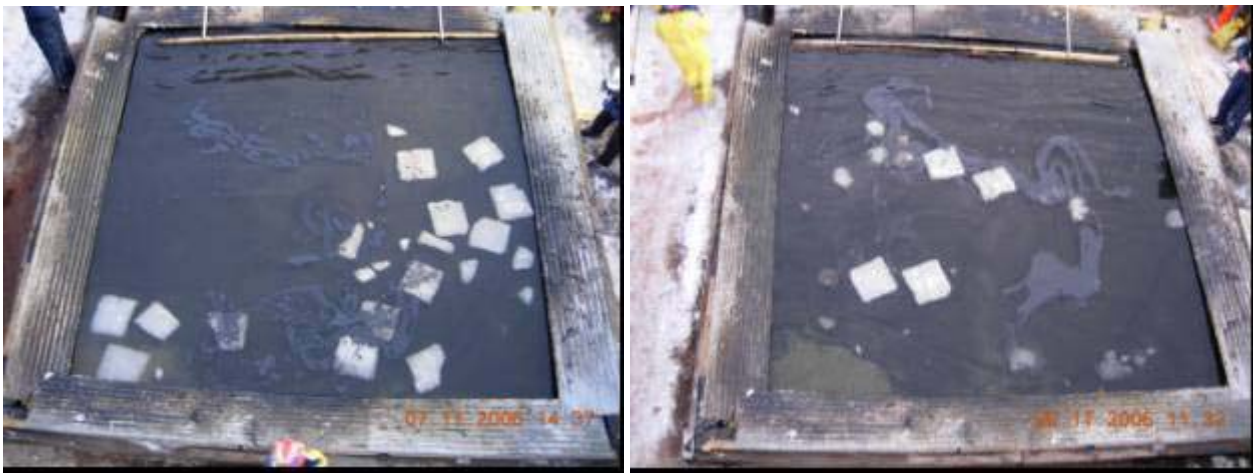
Figure 49: 1-s waves breaking up 7.5-L slick in test 16 (left) vs. 2-s waves in test 17 (right).
