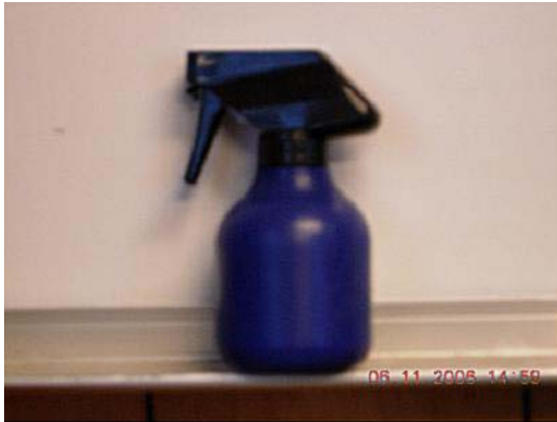
Figure 22: Spray bottle used to apply herder at Ohmsett.
