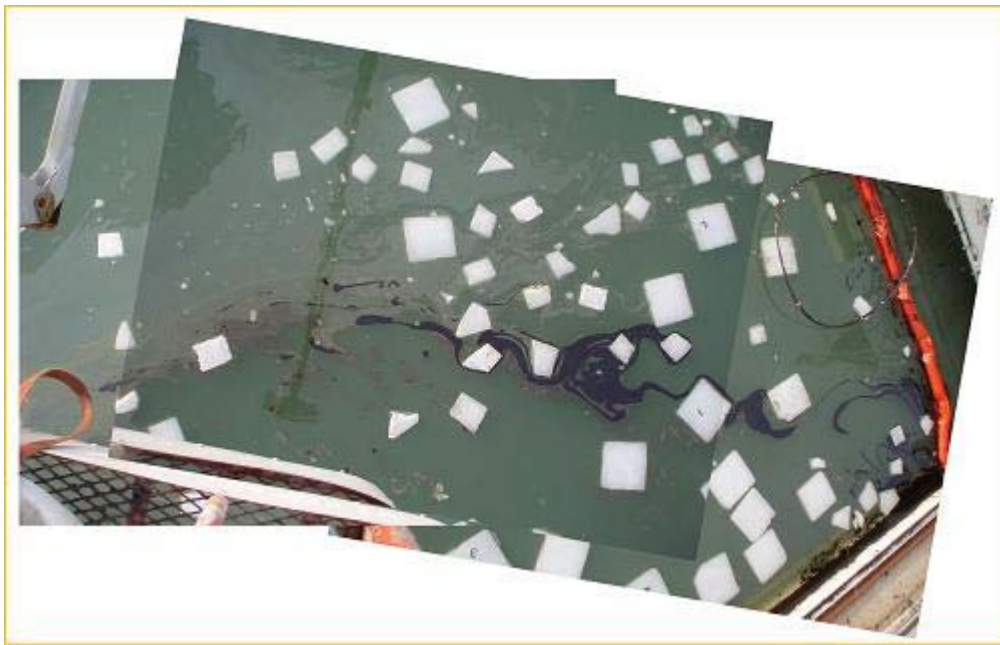
Figure 21: Composite picture of Test 5 oil slick used for area analysis.
