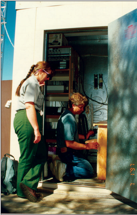
Air quality technicians at Yosemite National Park perform routine servicing on air quality monitoring instrumentation. Periodic training of park personnel in the proper operation of air quality monitoring equipment is part of the NPS' quality assurance program.
