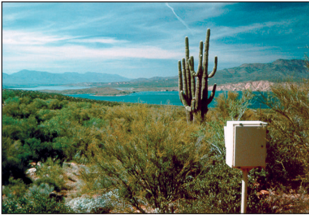
Scene monitoring camera system at Tonto National Monument, Arizona. The photographic documentation of how scenic views associated with national parks are affected by air pollution has been a very effective tool in the regulation of air pollutants at the national level.
