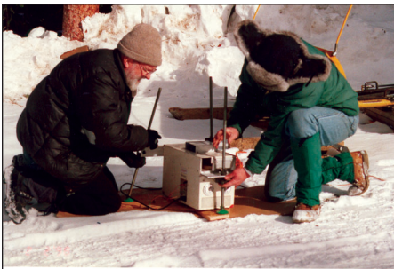
University of Denver researchers measure snowmobile emissions at Yellowstone National Park. Snowmobiles emit significant amounts of carbon monoxide and hydrocarbons during the 3 months that they are allowed in the park. Between 60,000 and 70,000 snowmobiles enter the park each winter.
