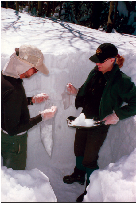
NPS employees collect snow samples in the Rocky Mountains to determine the amount of air pollutants deposited throughout the winter.
