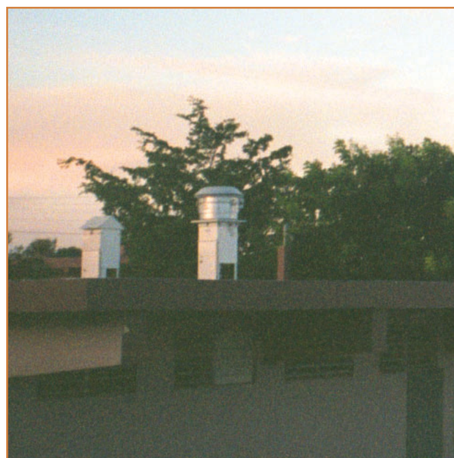
For the last 3 years, the Puerto Rico Environmental Quality Board has been measuring air pollution in two Vieques neighborhoods. This picture shows a sampling device in Esperanza.
