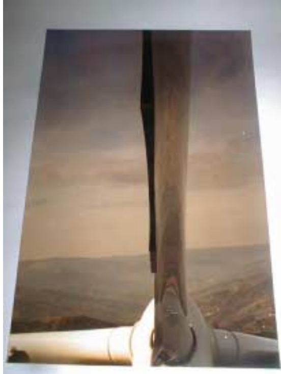
Figure 7. IVPC/Vestas blade damage
