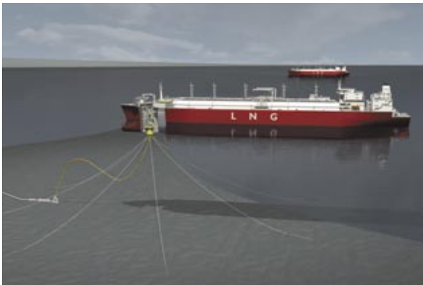
The proposed offshore LNG terminal in Massachusetts will be equipped with a 35-foot-high undersea buoy (Left). The buoy will serve as the anchor system for specially modified LNG tankers that incorporate onboard equipment to vaporize the liquid, which is piped to shore.
