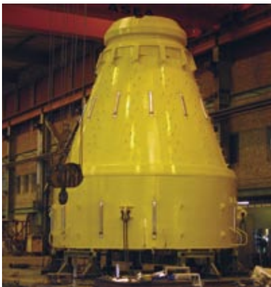
The proposed offshore LNG terminal in Massachusetts will be equipped with a 35-foot-high undersea buoy (Left). The buoy will serve as the anchor system for specially modified LNG tankers that incorporate onboard equipment to vaporize the liquid, which is piped to shore.
