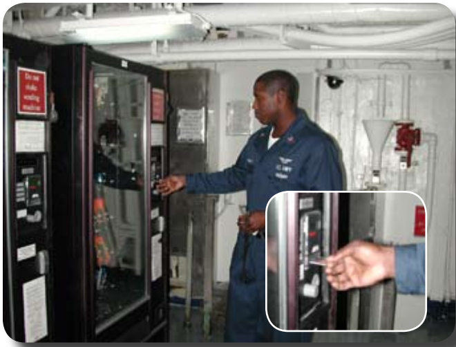
Card acceptance device (CAD) is loaded in vending machines to allow Navy Cash card to be used.
