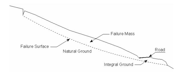
**Figure 2:** Failure of a large lateral extent of natural ground. While the failure mass threatens or otherwise impacts an eligible facility (the road) that portion of the natural ground integral to the support of the facility is small relative to the total failure mass of natural ground. Restoration of the large area natural ground along the failed slope would not constitute an eligible component of work.
