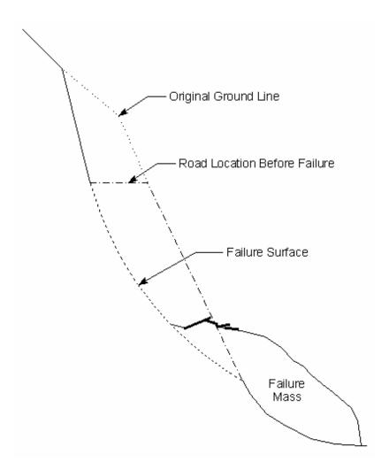
**Figure 3**: Failure of a slope along a road constructed by excavating into a hillside. In this case it may be more cost-effective to pursue other options under the Public Assistance Program.
