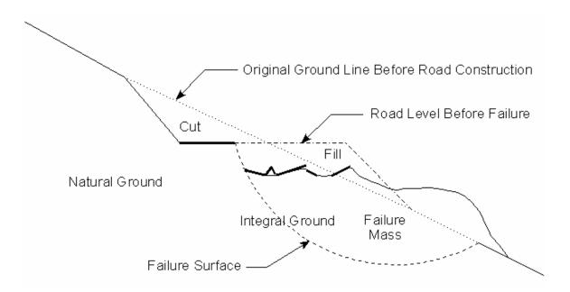
**Figure 1:** Slope failure in a typical cut-and-fill road section, illustrating the failure mass and the concept of integral ground beneath the facility. Restoration of integral ground in this case would constitute an eligible component of work required to repair the road, and would involve excavation slightly beyond the limits of the failure surface.
