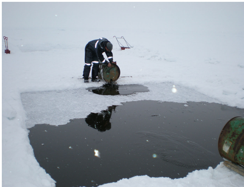
Figure 6-2 Sintef personnel pouring oil into the spill containment area for the oil under snow GPR field experiment in April 2008.
