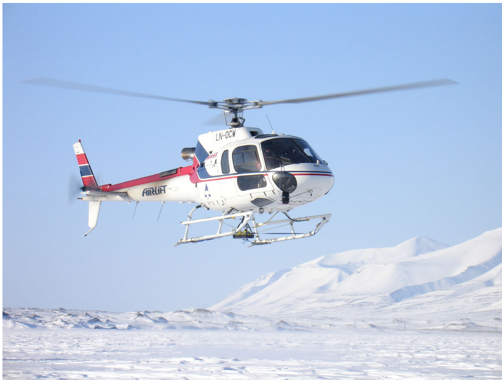
Figure 6-3 Photograph showing the 1000 MHz shielded antennas suspended from the cargo hook of the helicopter.
