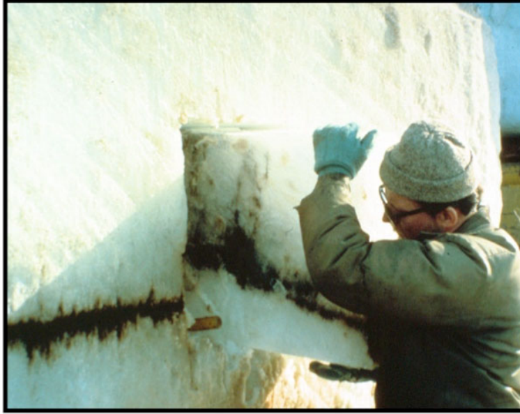
Figure 2-2 Oil encapsulated in ice during an experimental spill in Alaska. Photo: A. Allen
