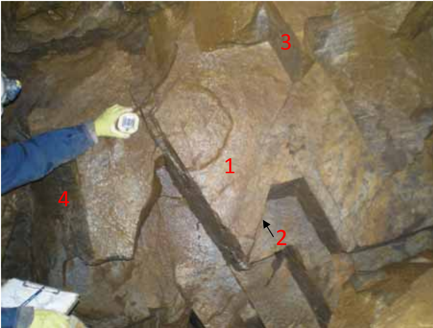
Figure 5: Looking south at four fracture sets exposed in the South Room. All fractures in this photograph fall into one of the three fracture sets determined from the rose diagrams. 1: Flat face oriented 261/76N 2: 350/77 E 3: 151/55 SW 4: 130/75 SW
