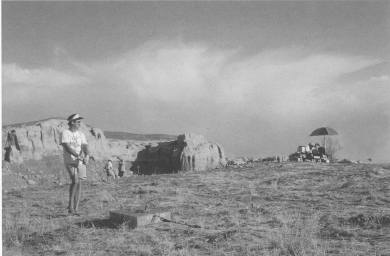
Figure 2. Collecting GPR data with 300 MHz antennas at the Bluff Great House site, Utah. Radar energy is transmitted from the base station (under umbrella on the right) to the antennas. The reflected data from below the surface is re-transmitted back to the base station in the same cable where it is recorded and can be viewed on a computer screen.
