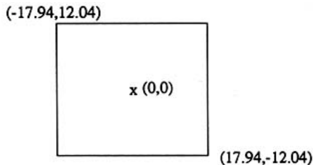
Figure 3 1. Coordinates for corners or 35 mm film
