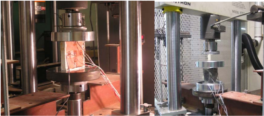
Figure 60: The hydraulic displacement controlled testing of tile and mortar unit.
