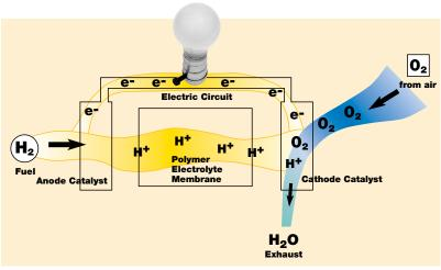
electrolyzer uses energy from solar or wind units to split water into hydrogen and oxygen atoms. The hydrogen atoms can then be stored in tanks and used later in a fuel cell to produce clean, quiet power when the sun goes down or the wind stops blowing.
