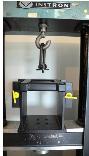
Figure 3.7: Instron machine with testing frame
