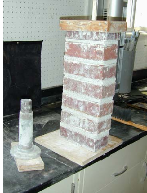
Photo 6 – Mortar joints in fabrication with drop hammer. ASTM C1329.
