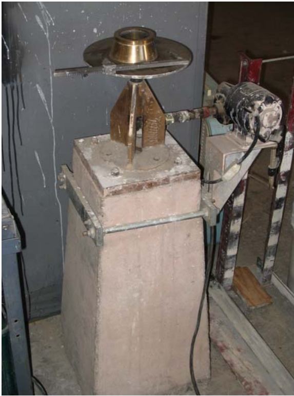
Photo 1 – Flow table as per ASTM C 230.
