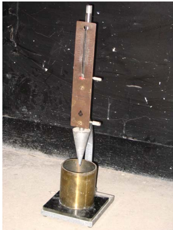
Photo 4 – Vicat penetrometer ASTM C 780.
