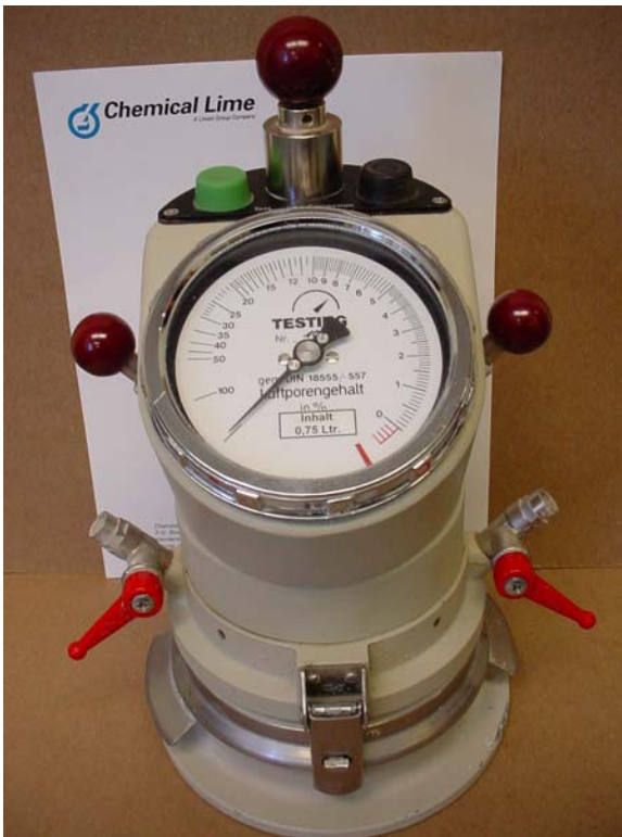
Photo 3 – Air pail apparatus as per ASTM C 231.
