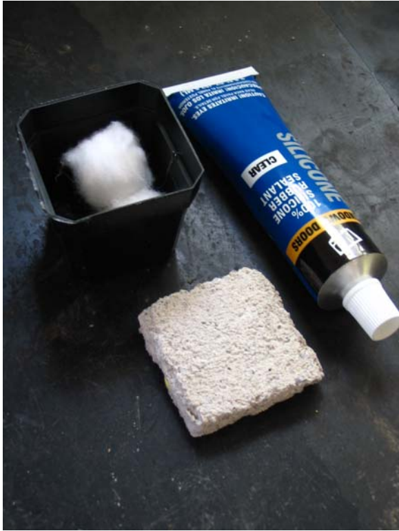
Photo 10 - WVT test cup preparation showing test cup, cotton ball to prevent splashing of water, ½ inch mortar sample and silicone caulk.
