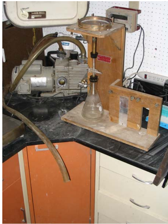
Photo 2 – Vacuum apparatus used for determination of water retention ASTM C 1506.
