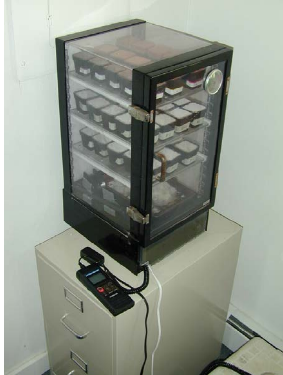
Photo 11 – WVT chamber using magnesium nitrate soluble salt to mediate RH.
