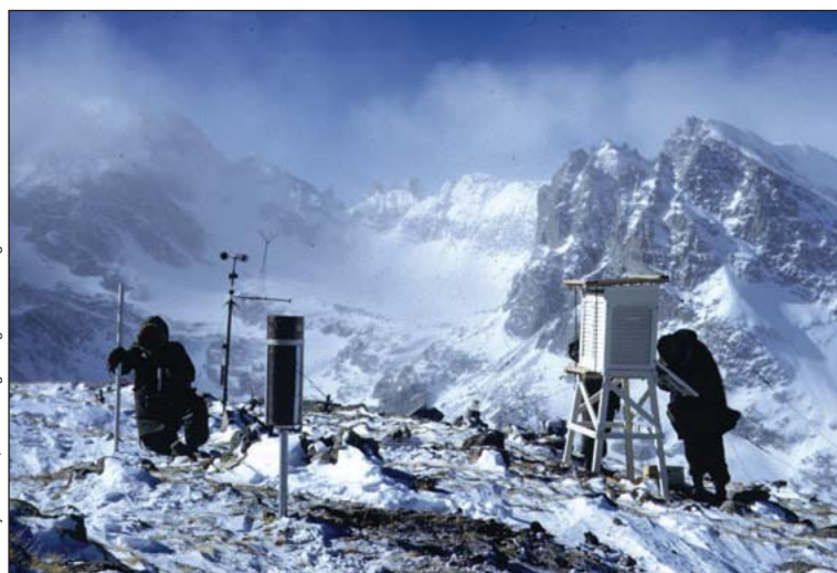
Figure 4. To apply a critical loads approach, scientists must know the current levels of atmospheric sulfur and nitrogen deposition. These values can be difficult to quantify, especially in high-altitude settings, such as that pictured here at Niwot Ridge, CO, where wind and extreme cold test the ability of instruments to document atmospheric loads. Photo taken at the D-2 Meteorological Station, ca 1953.
