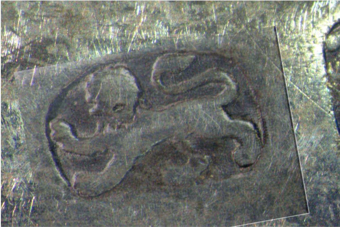
Figure 7. A recovered acoustic image of a worn-off lion hallmark overlaying a digital image of an identical hallmark from the same set of teaspoons
