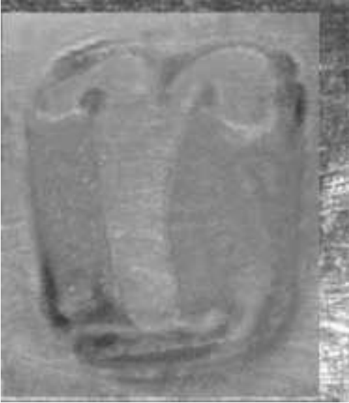
Figure 8. Recovered acoustic images of the date letter 'r' overlaying a digital image of a visible 'r' hallmark from the same set of teaspoons
