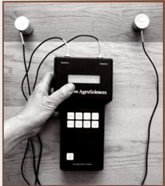
Figure 6. The acoustic emission detector (AED) recorded sound waves that were generated when wooden fibers were broken by termite mandibles, and was used to measure termite feeding in wood.
