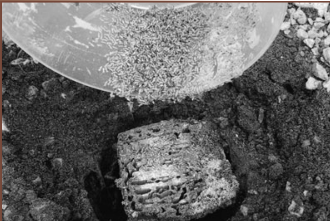
Figure 4. The field trials used underground (A) and aboveground (B) monitoring stations to measure termite activity at several historic sites.
