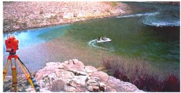
Hydrographic surveys determine the amount of sand stored in the channel.
