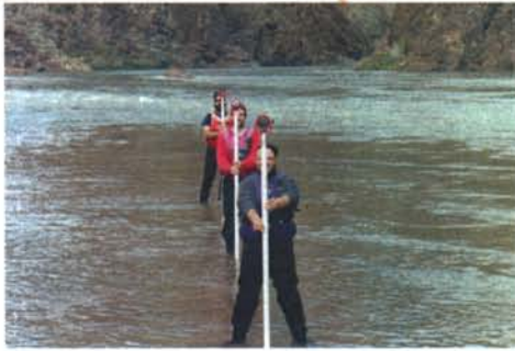
Topographic surveys determine the amount of sediment stored on sand bars.
