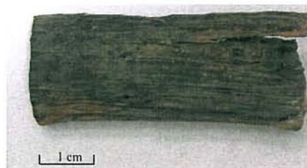
Figure 19. Sample 30d split due to air drying.
