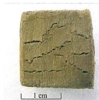
Figure 20. Cracking exhibited by MD sample 89.
