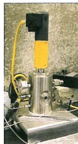
Figure 12. The supercritical reactor chamber and impeller head (yellow).
