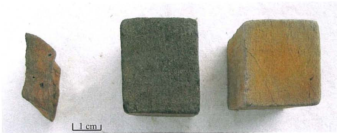
Figure 49. Treated MG-B blocks. Left to right- air-dried sample 17, freeze-dried sample 6, supercritical-dried sample 3.
