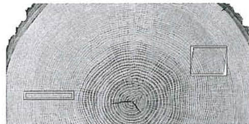
Figure 22. Orientation of subsamples in context of a log. with expected warp as a result of drying.
