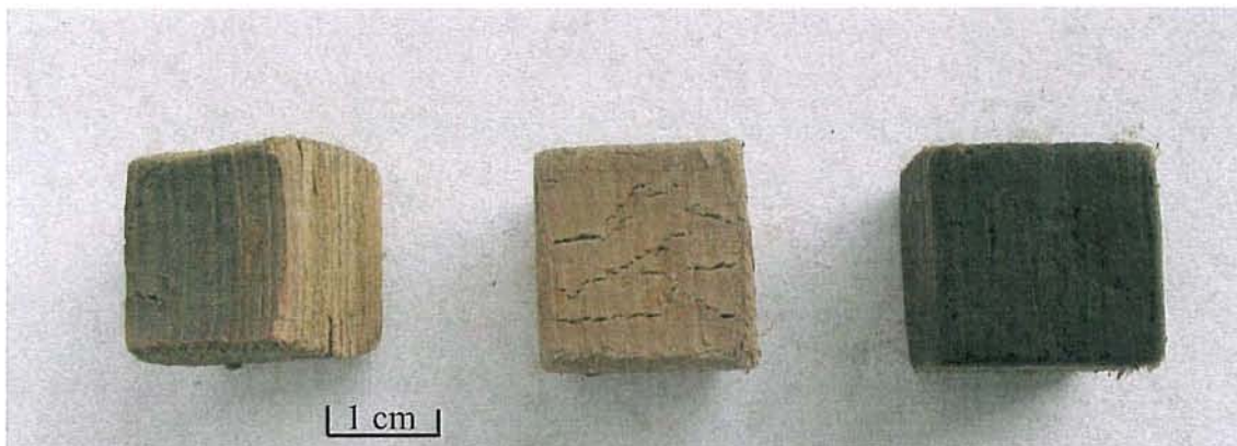
Figure 51. Treated MD blocks. Left to right- air-dried sample 83, freeze-dried sample 88, supercritical-dried sample 87.
