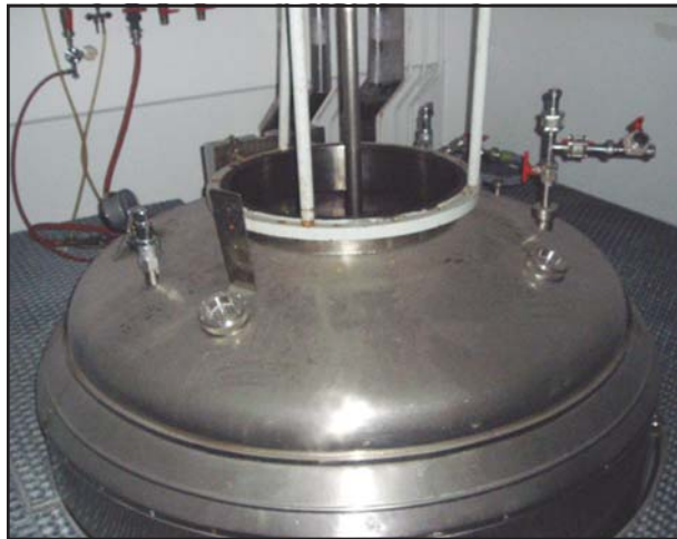
Figure 9. Sign at the entrance to FMDV “Almanai” (top left), vial of vaccine dating from 19 October 1983 (top center), and a main production fermentor (top right). Top plate of 3,500-liter bio-reactor (bottom left), and 236-liter bio-reactor (bottom right).
