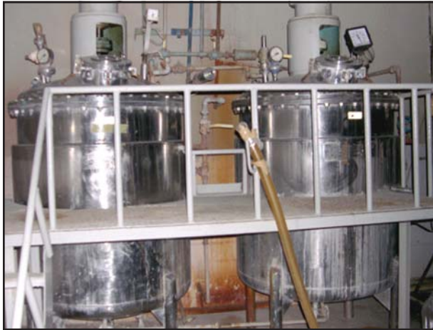
Two 1,000-liter, stirred, jacketed vessels suitable for use as fermentors for the growth of bacterial BW agents.
