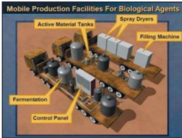
Figure 11. Truck-mounted BW production unit—based on source reporting.
