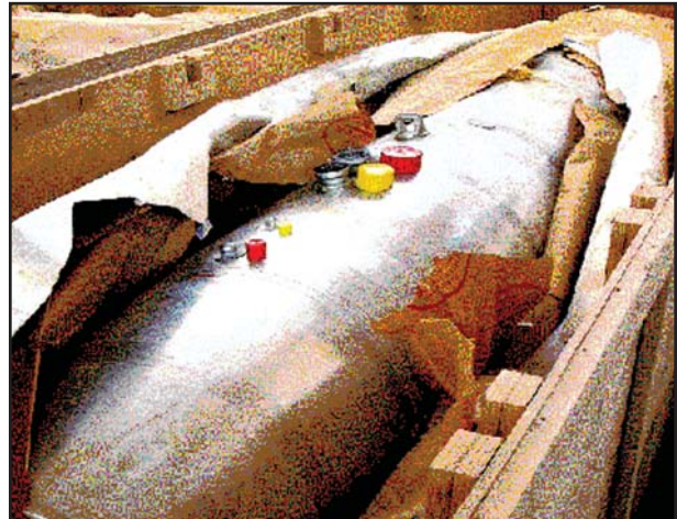
Al-Asad: new Mirage FI drop tank (France).
