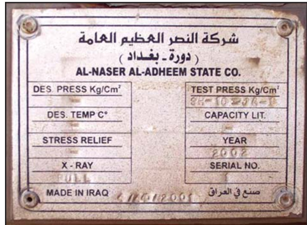
Figure 3 (b). Trailer 1 data plate on reactor vessel.
