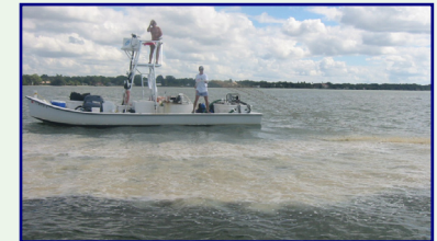
Control by clay flocculation being tested in the field. This method has shown effectiveness for controlling blooms under certain conditions. (Photo: Richard Pierce, Mote Marine Laboratory)
