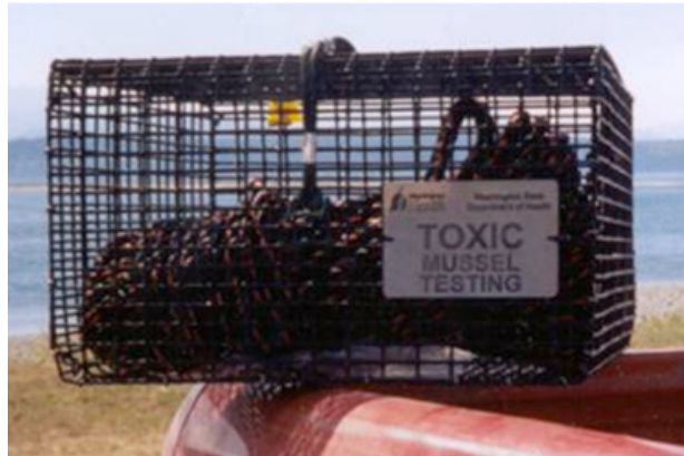
A mussel cage used in the Washington Department of Health's Sentinel Mussel Biotoxin Monitoring Program. Photo: Liz Cox-Bolin and Frank Cox
