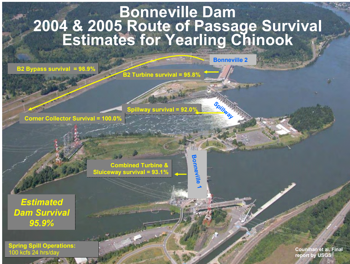
Figure A-5. Route-Specific Dam Survival Estimates for Yearling Chinook Salmon for 2004 and 2005
