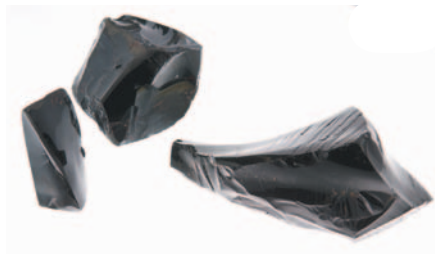
Stabilization of nuclear weapons byproducts in glass
