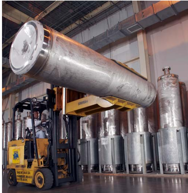
DWPF has poured over nine million pounds of vitrified waste into more than 2,200 canisters.
