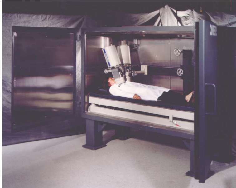
Figure 2-3. Low Energy Germanium (LEGe) Based Lung Counter. This instrument is designed to maximize sensitivity for internally deposited U, Pu and Am isotopes. Germanium is used to provide the system with the ability to resolve the differences between photons which are close in energy to each other. (Photograph courtesy of Canberra Nuclear/Packard BioScience Co.)
