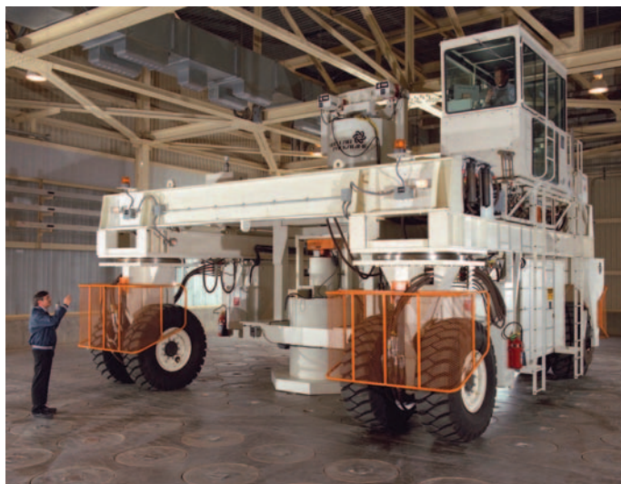
▲ The Shielded Canister Transporter moves filled canisters into the Glass Waste Storage Building.
