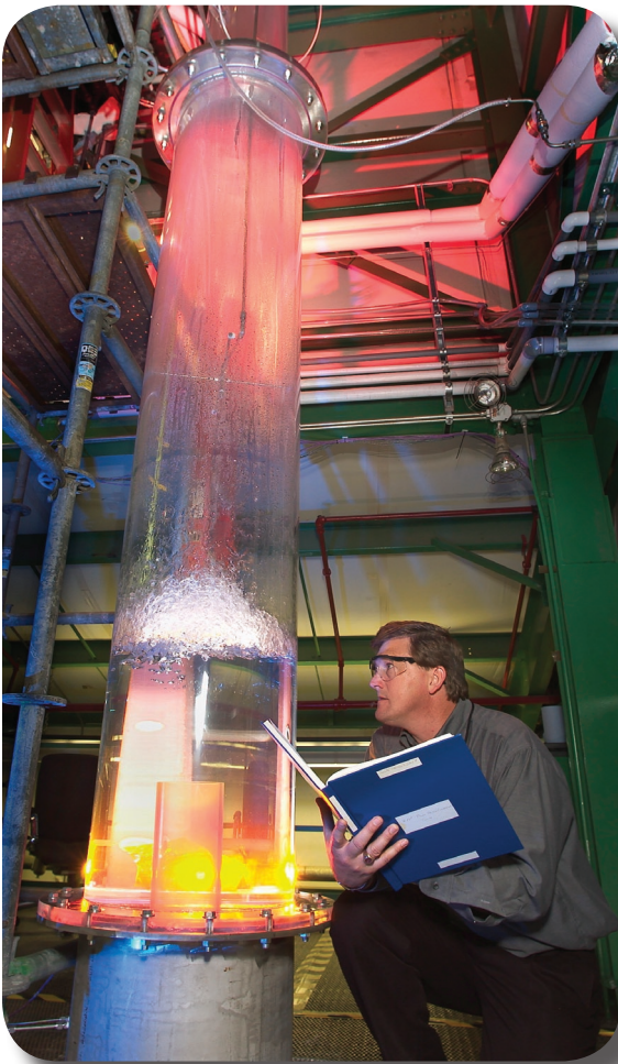
SRNL conducts pilot-scale testing of Hanford's waste pretreatment system, including the evaporator system
