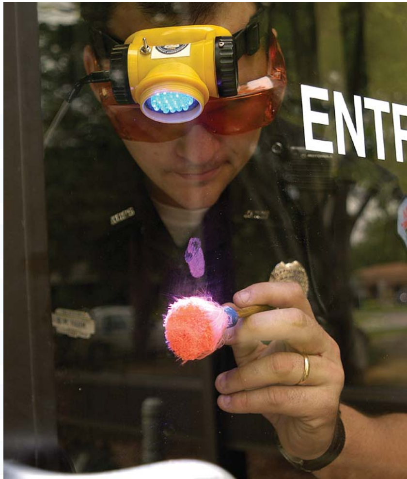
An Aiken Public Safety officer uses the SRTC-developed BritePrint to reveal fingerprints and other markings that may have gone undetected using conventional methods.
