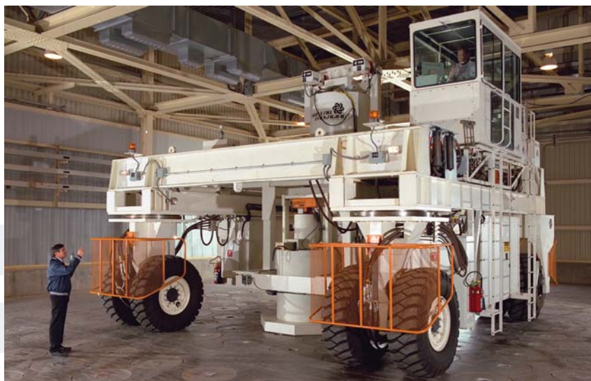
DWPF's shielded transporter maneuvers into place in the Glass Waste Storage Building.
