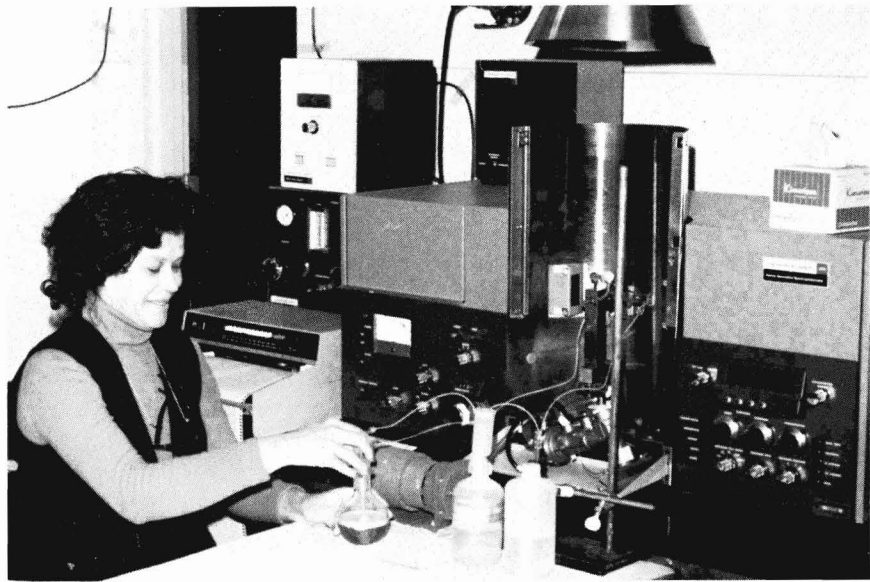
Chemist Alice Hall is determining mercury in fish samples, using an atomic absorption spectrophotometer (Utilization Research Division photo, Seattle, 1967).
