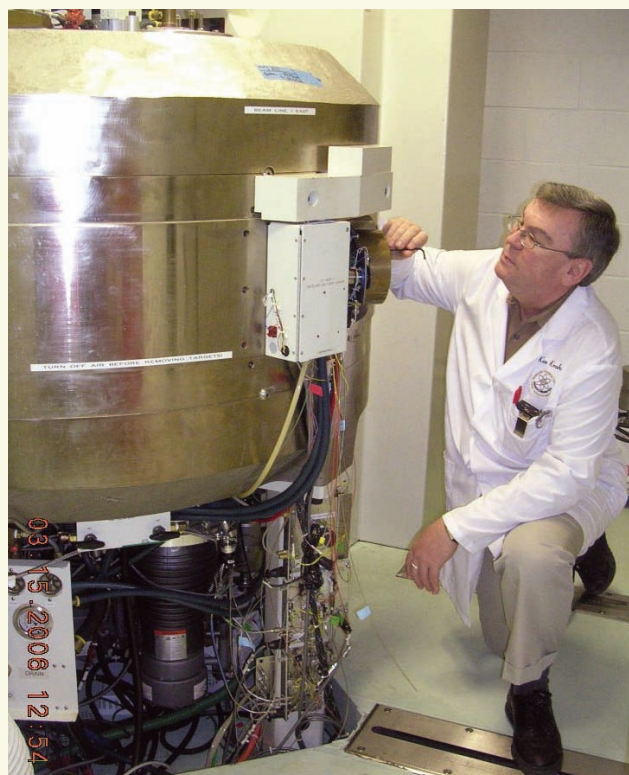
■ Kenneth Krohn prepares to create radioactive tracers in a state-of-the-art cyclotron acquired through an HEI grant. The tracers are used primarily for cancer imaging in patients.
