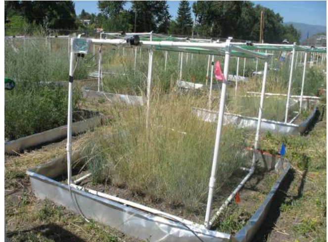
Research plots with automated precipitation covers to study effects of climate change on weed invasion and biocontrol.
