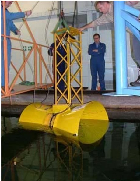
Duct inlet diameter for 2 MW unit is 25 m
