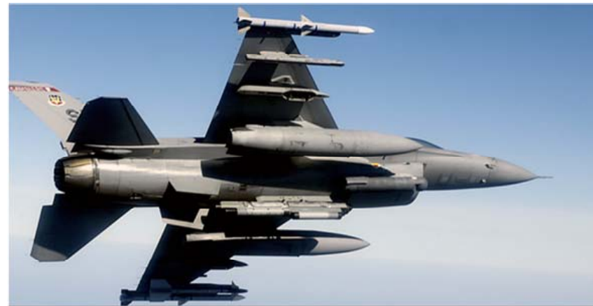
A U.S. Air Force F-16 Fighting Falcon aircraft flown by Maj. Marc Himelhoch from the 77th Fighter Squadron, Shaw Air Force Base, SC., looks for simulated targets and hostile aircraft during exercise Operation Iron Thunder. The aircraft is armed with AIM-120 Advanced Medium Range Air-to-Air Missile (AMRAAM) missiles on each wing and an AIM-9M Sidewinder missile (left wing).
