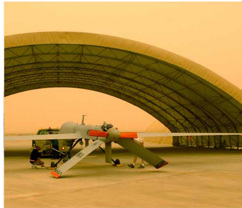
An MQ-1 Predator unmanned aerial vehicle is hooked up to be taxied for maintenance after flying a mission at Balad Air Base, Iraq. The Predator provides armed reconnaissance, airborne surveillance and target acquisition in Iraq.
