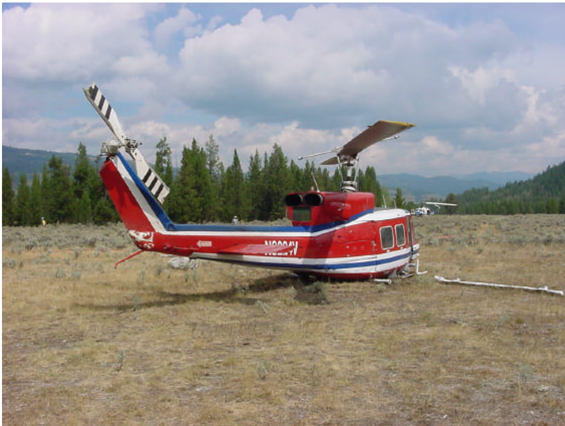
Bell 212 sitting on belly after skid failure
