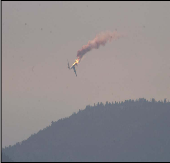
PB4Y-2 airtanker upon wing separation.
