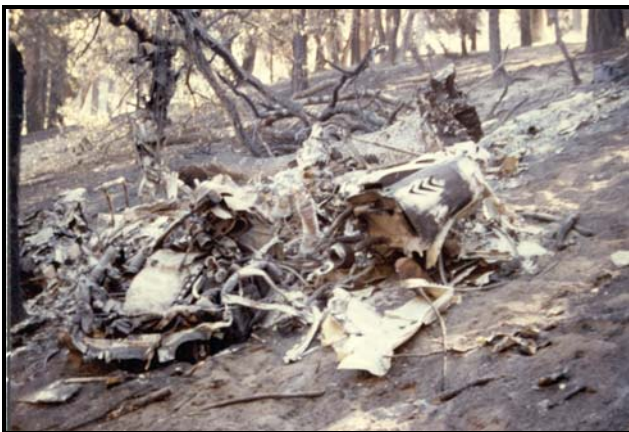
Baron wreckage looking southwest. On the left is the left engine, upside down. Right of the left engine is the nacelle (air scoop is open, in flight position) indicating the air conditioner was on. Tail section with cables hanging over tree limb.
