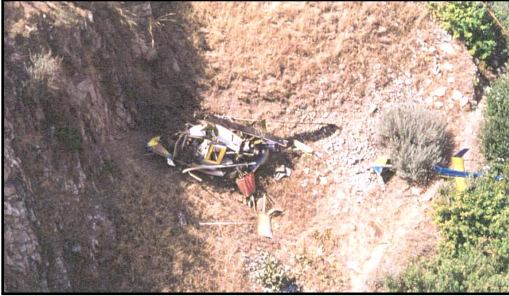
Close-up of Bell 206LI mishap site. Tail rotor actually found under nose and moved to permit access to cockpit.
