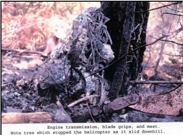
Engine transmission, blade grips, and mast of Bell 206LIII.
