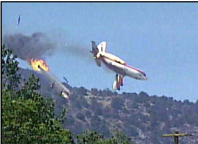
C-130A airtanker after its wings separated from the fuselage.
