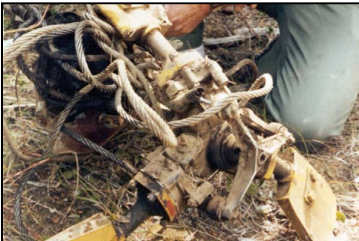
Tail rotor system with entangled cable was found 250 feet south of the main wreckage. All 100 feet of the cable was intact and found at this point.
