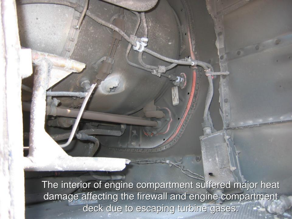
A post-landing examination of the helicopter revealed that a puncture from the inside out existed in the hot section of the right engine. The engine compartment, engine deck, firewall, cowling attachment point, and other accessories on the right side of the helicopter sustained damage.
