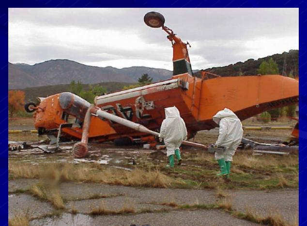
The snorkel became lodged to the tank between the tank band and the lifting eye. The nose of the aircraft went down and the pilot pulled back on the cyclic and applied power
