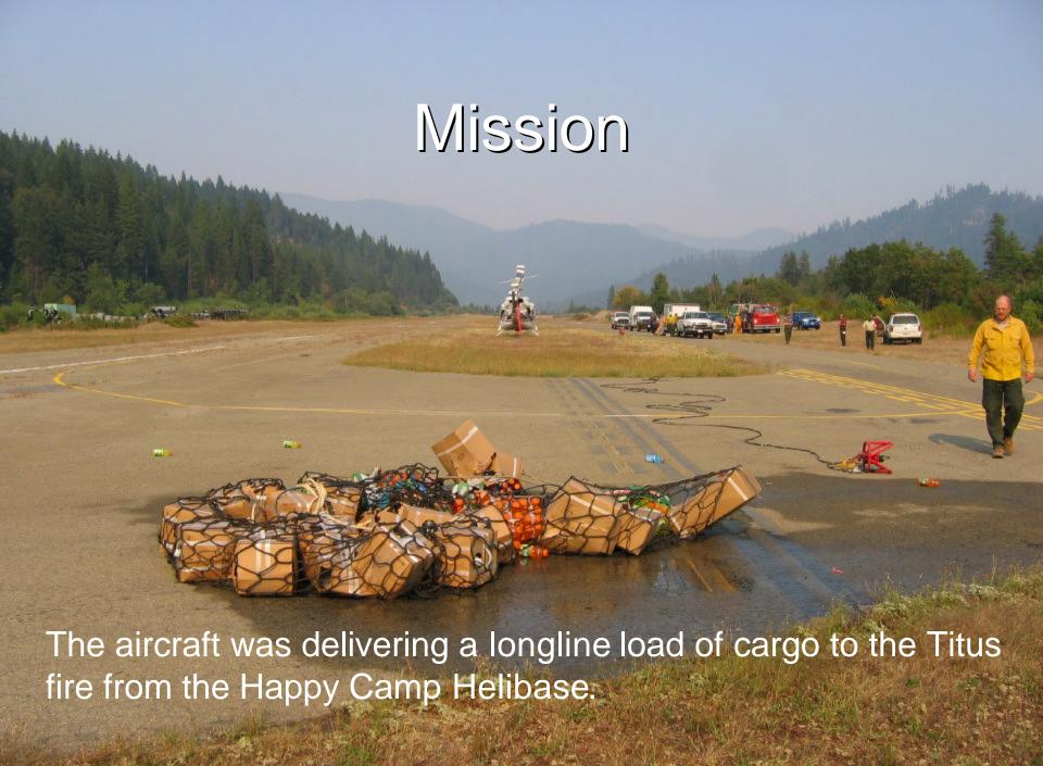
Just after departing the Happy Camp Helibase the pilot smelled smoke. He immediately turned back towards the base and called on the radio to ask if they could see smoke from the aircraft. He then got an engine fire warning light on the annunciator panel. Pilot quickly got to a safe location and jettisoned the longline, pulled the engine fire extinguisher and landed the aircraft.
