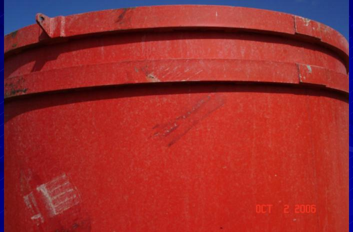
The aircraft continued to spin (2nd rotation), the tail rotor head contacted the retardant tank a second time breaking off the 90 degree tail rotor gearbox, and also breaking off the last 1/3 of the tail boom.
