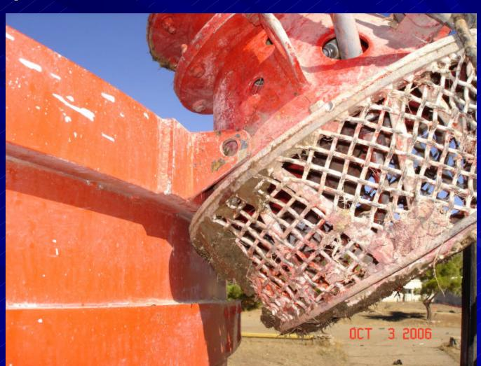
The nose of the aircraft came up but was in a left bank with a high nose up attitude, the tail stinger contacted the ground and the aircraft spun around to the left. On this first rotation, the tail rotor blades contacted the retardant tank; two of the blades (symmetrically) depart the aircraft
