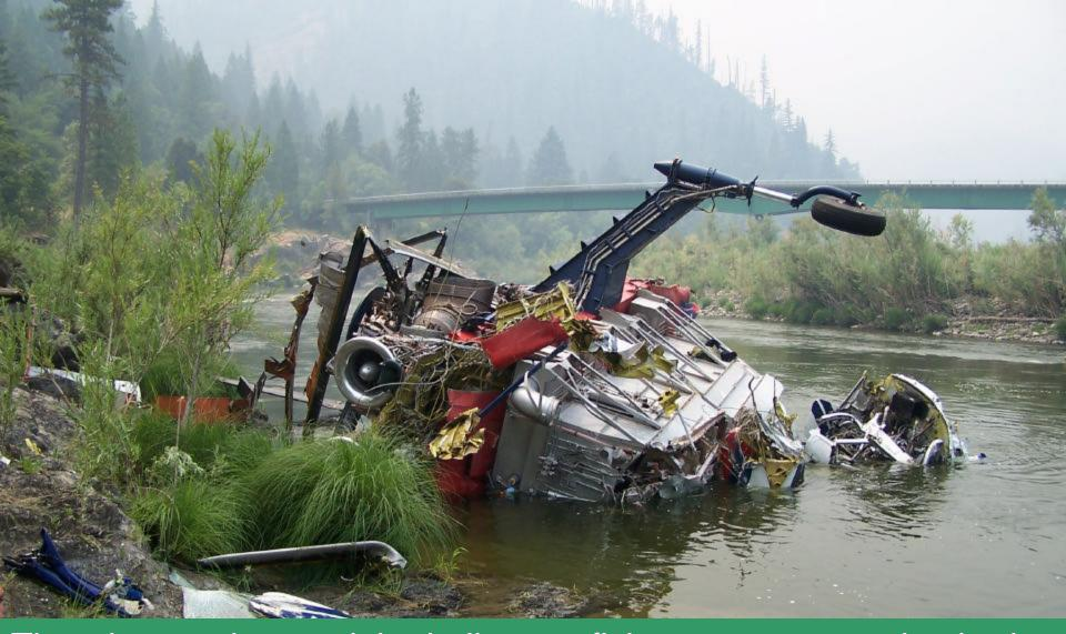
The witness observed the helicopter flying over a stone riverbed toward the Independence Bridge. He then noticed a large piece fall off the helicopter, which was later identified as the tail rotor gearbox with three of the four tail rotor blades attached to the hub.
