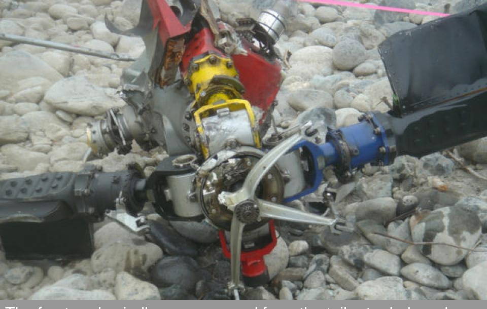
The fractured spindle was removed from the tail rotor hub and shipped to the National Transportation Safety Board Materials Laboratory in Washington, D.C., for further examination.
