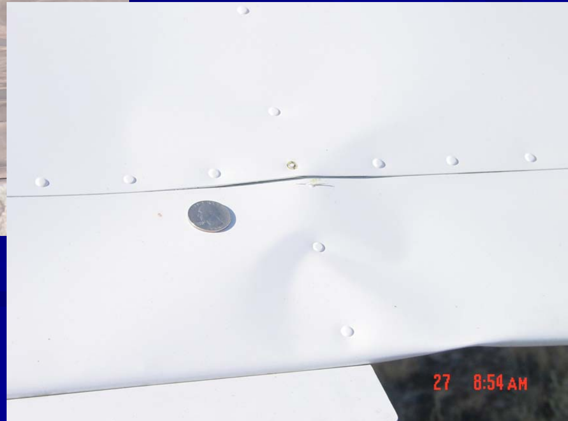
Bent ribs and wrinkled aileron
