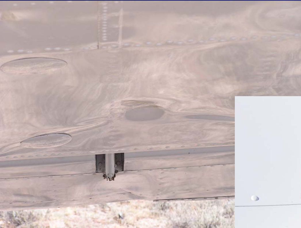
Bent ribs and wrinkled aileron
