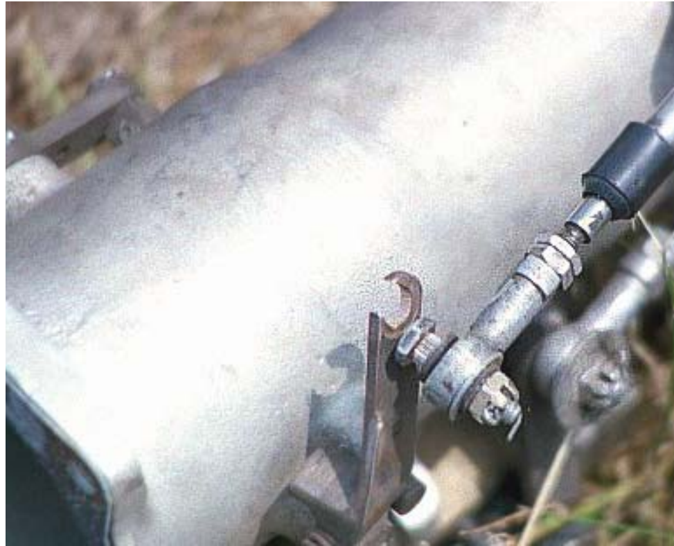
Throttle linkage failed in flight
